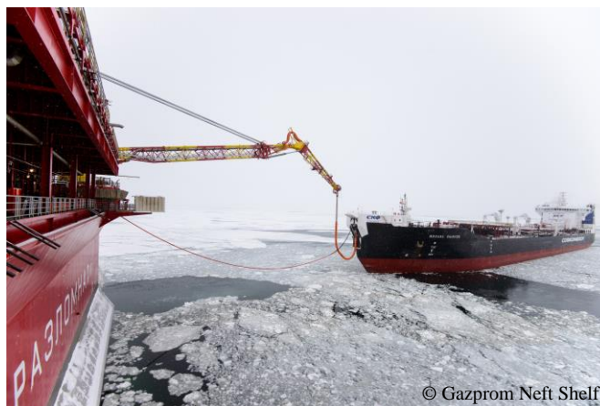
Figure 4.21 In 2010, Sovcomflot, the world's number one operator of the Arctic shuttle tankers, received two 70 000 tonnes deadweight double acting ice-class tankers, Mikhail Ulyanov and Kirill Lavrov , built at the Admiralty Shipyards in St Petersburg. In 2015, these tankers were serving Prirazlomnoye project delivering Arctic crude oil from the Pechora Sea to the Western Europe. Photo: Mikhail Ulyanov receives oil from Prirazlomnaya platform.
