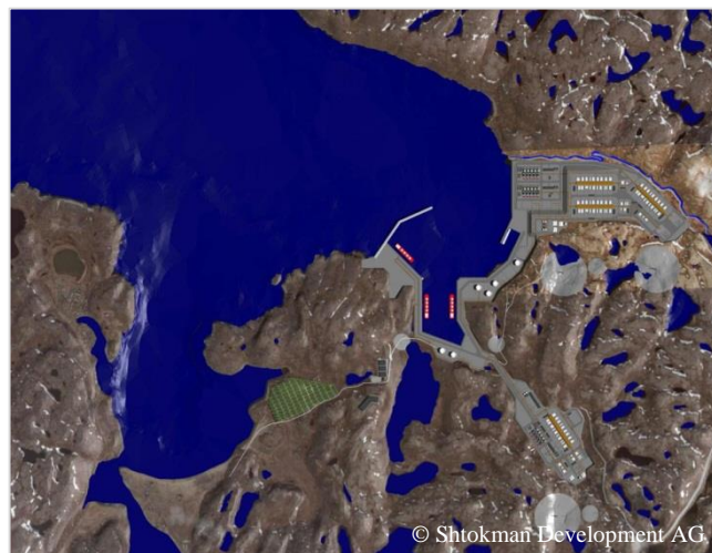
Figure 4.79 The scheme-view on the facilities to be built in Zavalishina Bay near Teriberka within three phases of the Shtokman project with the overall annual production capacity of about 23 million tonnes of liquefied gas.
