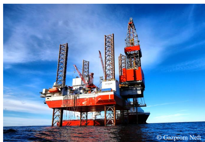
Figure 3.14 GSP Saturn jack-up rig (photo) of the Romanian company GSP Offshore worked in the Pechora Sea for Gazpromneft-Sakhalin drilling and testing an exploration well at Dolginskoye field during summer 2014.
