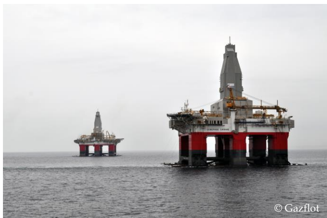
Figure 3.18 Polyarnaya Zvezda (Polar Star) and Severnoye Siyanie (Northern Light) semi-submersible floating drilling rigs were initially constructed for Shtokman project. In 2014, both rigs worked on Sakhalin-3 project in the Okhotsk Sea. Photo: two rigs on the road.
