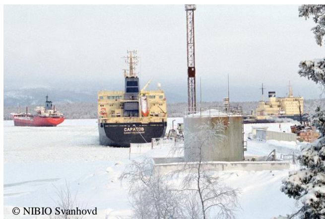
Figure 4.75 In 2002, the port of Vitino started year-round operations. During winter navigation, oil was offloaded to 20 000 tonnes ice-reinforced tankers, and shipment operations were assisted by icebreakers.
