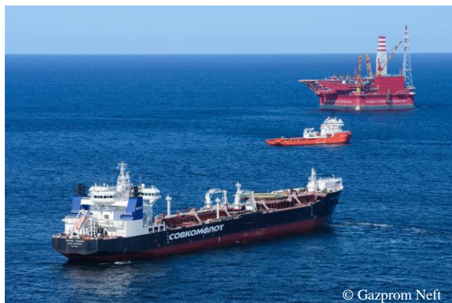
Figure 6.3 70 000 deadweight tonnes double acting Arc6 ice-class tankers Mikhail Ulyanov and Kirill Lavrov were built at Admiralty Shipyards in St. Petersburg and delivered to Sovcomflot in 2010 for Prirazlomnoye project. In 2014, Prirazlomnaya platform started to offload Arctic crude oil for export.
