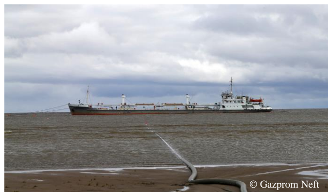
Figure 4.47 In August 2014, Gazprom Neft ran the first operation on offloading Novy Port crude oil in the Ob Bay for sea transportation. Photo: Lenaneft river tanker receives Novy Port crude oil in the Ob Bay via a temporary pipeline.
