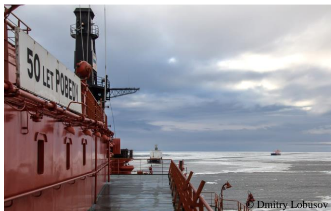
Figure 4.68 During winter navigation, vessels are receiving icebreaking assistance to pass through ice-covered waters of the White Sea. Photo: 50 Let Pobedy piloting bulker Zapolyarye and tanker Weichselstern on their way from Arkhangelsk to open waters of the Barents Sea.
