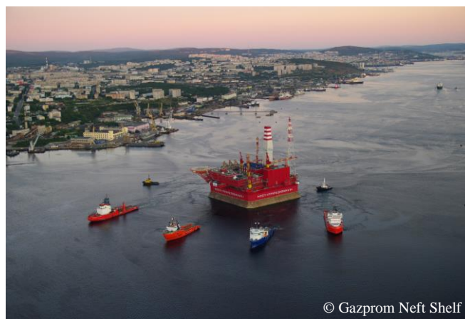
Figure 4.59 In August 2011, when ballasting and modernisation works at the Factory # 35 were completed, Prirazlomnaya platform was towed from Murmansk to Prirazlomnoye oil field in the Pechora Sea (photo).
