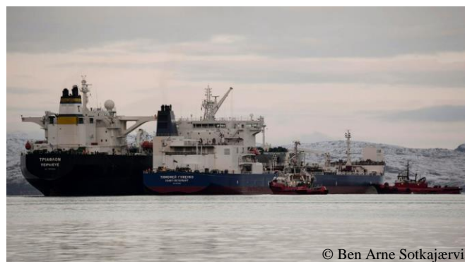
Figure 4.98 Norterminal started oil transshipment operations in Bøkfjord in October 2014 using 165 000 tonnes deadweight Triathlon to transfer oil between shuttle and export tankers. Photo: Timofey Guzhenko delivers first cargo of crude oil to Triathlon .
