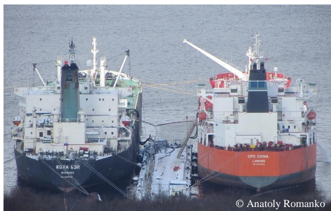
Figure 4.85 51 700 tonnes deadweight CPO China receives heavy fuel oil from FSO Kola Bay at the terminal in Mokhnatkina Pakhta, March 2013.
