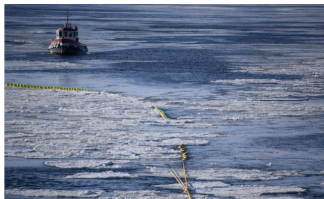
Figure 6.3 Testing of ice towing equipment for use in Arctic oil spill response (photo). Tests were performed by Viking Ice Consultancy, Norterminal and Egersund Group in Kirkenes area in June 2015.
