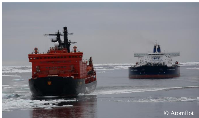
Figure 4.28. 162 000 deadweight tonnes tanker Vladimir Tikhonov loaded with 120 800 tonnes of gas condensate made the Northern Sea high-latitude path under pilotage of 50 Let Pobedy (photo) and Yamal in 2011.
