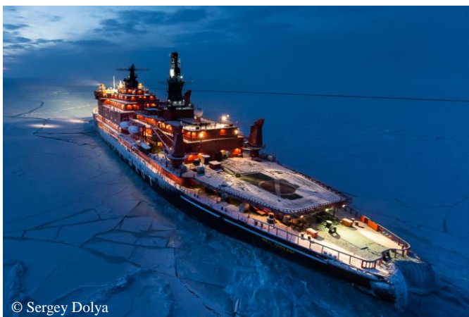
Figure 4.22 The Russian Arctic navigation is supported by a total of nine icebreaker liners, including five nuclear-powered ones. The biggest in the world icebreaker, 50 Let Pobedy , was completed in the Baltic Shipyard – Shipbuilding in St Petersburg in 2007 and delivered to state-owned Atomflot. Photo: 50 Let Pobedy at the North Pole expedition.
