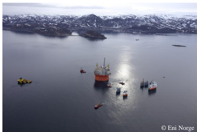
Figure 4.107 Floating, Production, Storage and Offloading unit (FPSO) built for Goliat started its voyage from South Korea to Norway in February and arrived Hammerfest in April 2015. Goliat FPSO should be put on stream and offload oil in 2016. Photo: Goliat FPSO floated off Dockwise Vanguard semi-submersible heavy lift vessel in the Barents Sea.
